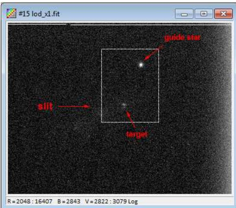
Open guide window with an adequate exposure time. Activate the slit mode **pressing SHIFT + click on guide window image** and press "Mark guide star" button. Move the cross-hair toward the guide star by clicking on proper border side of image until autoguide is engaged. The star is locked on cross-hair center.
