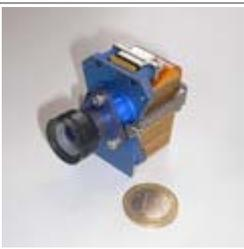
X-Cam was designed by Swiss company Micro-Cameras & Space Exploration. It is the latest in a series of miniature cameras built by the company for previous ESA missions including Proba-1, SMART-1 and Rosetta.
